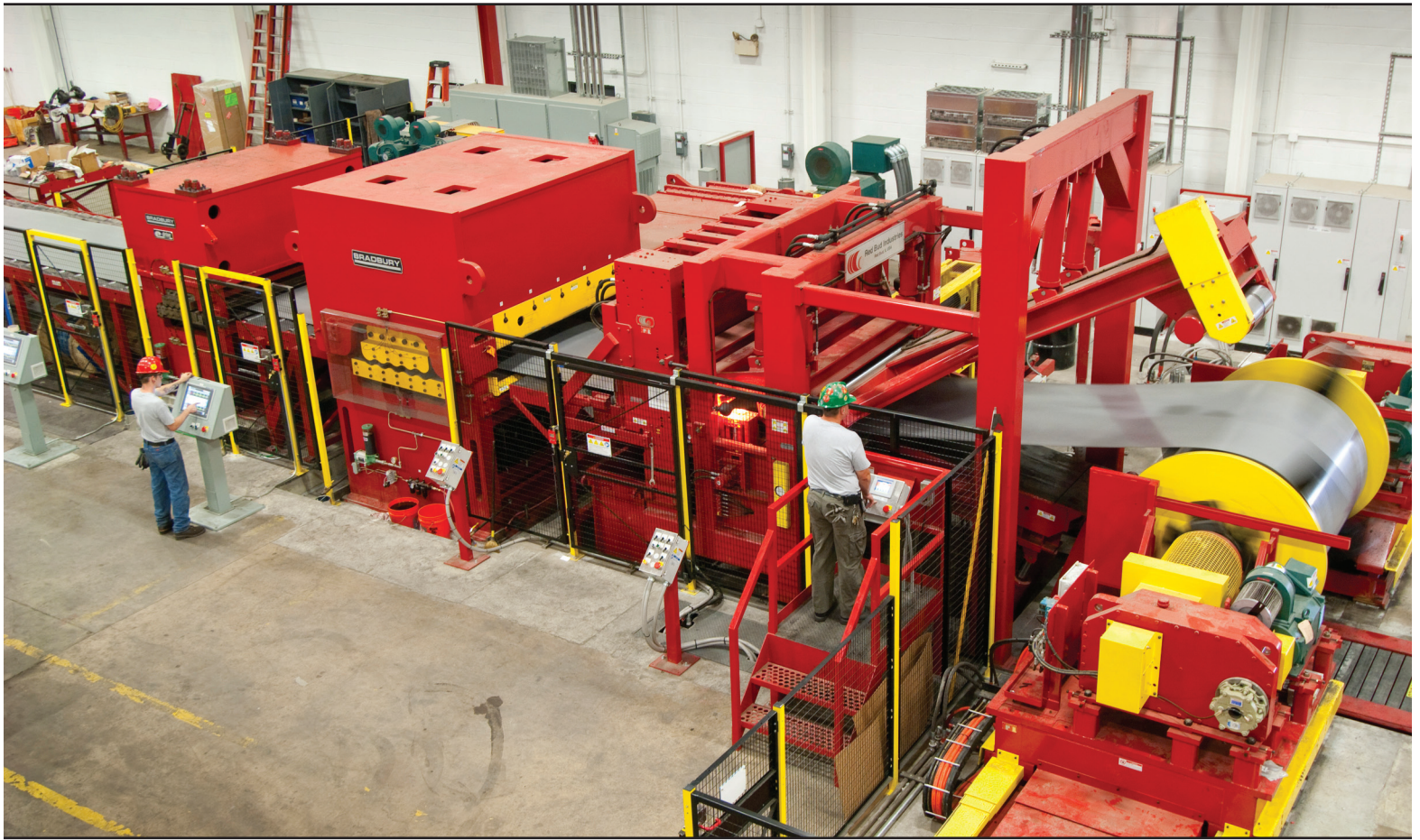
Processing begins with uncoiling and feeding material through a straightener into the Bradbury roller levels.
