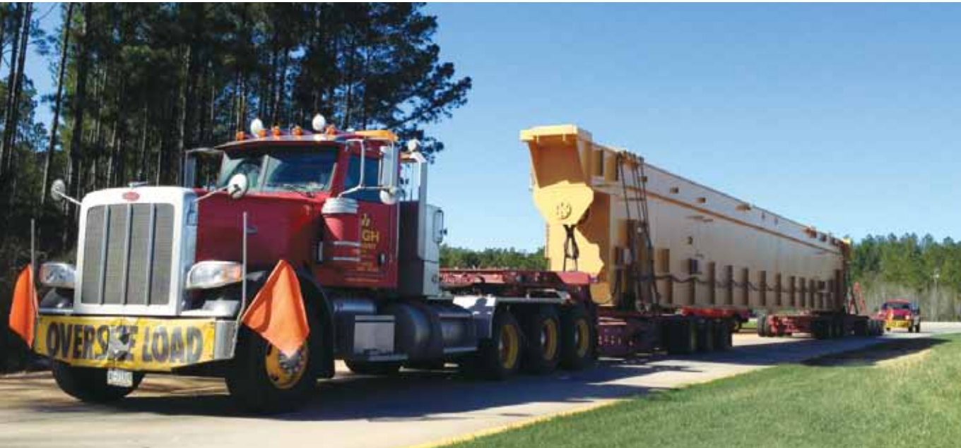
Top: A 75-ton, 91-foot-long bridge box girder makes its way to a construction site on the New Jersey Turnpike from High Steel Structures' Williamsport, Pennsylvania, facility in one day.
