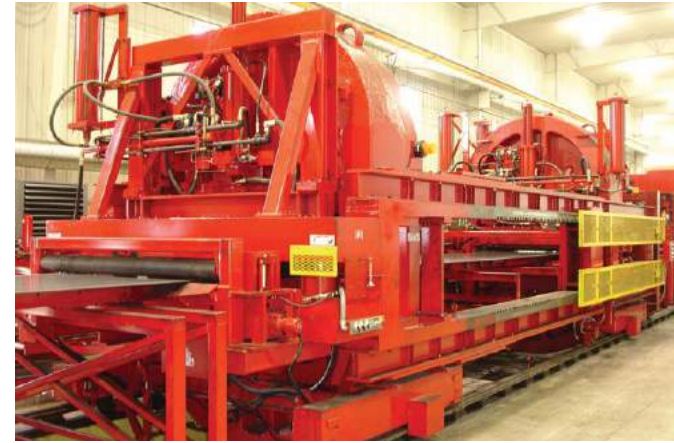
High Steel Service Center is the Mid-Atlantic region's only supplier of panel-flat, stress-free metal stock processed through a Red Bud Industries stretcher leveler.
