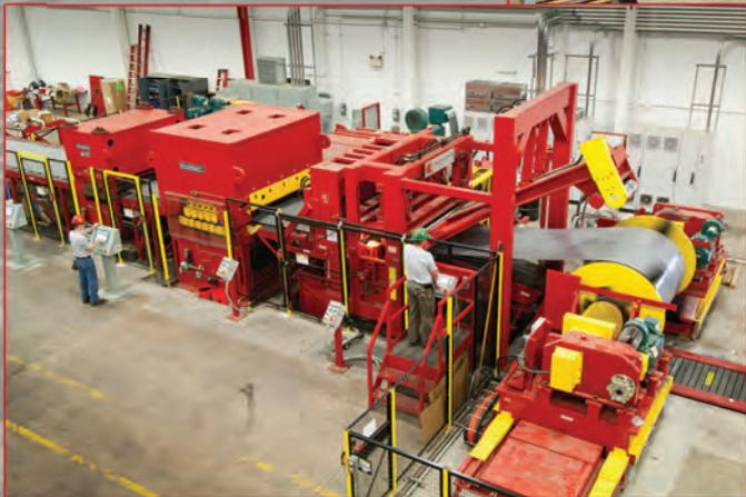
▶ HIGHSL processing begins with uncoiling and feeding material through a straightener into the roller levelers. Initial leveling by Bradbury roller levelers removes the majority of stresses, preparing the material for the Red Bud stretcher leveler.
