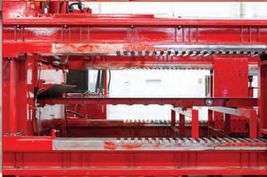
▼ A computer-controlled digital positioning system ensures reduced set-up time and precise control of the combined leveler operations.
