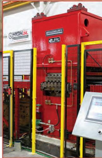
◀ The Bradbury eDrive roller leveler prevents bunching, increasing plunge of the entry rolls to obtain maximum yield of the material for more stretch and deeper penetration.
