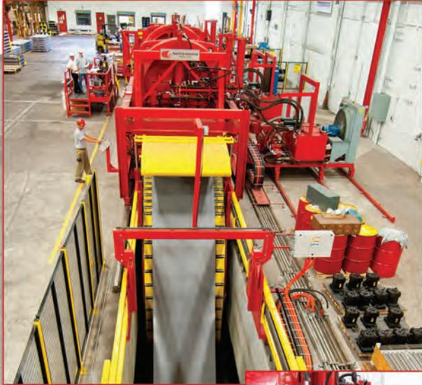
► Red Bud Industries' stretcher leveler technology precisely grasps the sheet or plate, up to one-half-inch thick, and stretches it past the material's yield point, removing all internal stresses.
